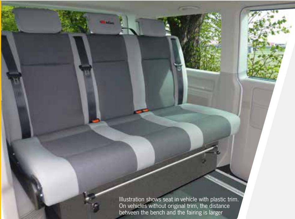
Illustration shows seat in vehicle with plastic trim. On vehicles without original trim, the distance between the bench and the fairing is larger
