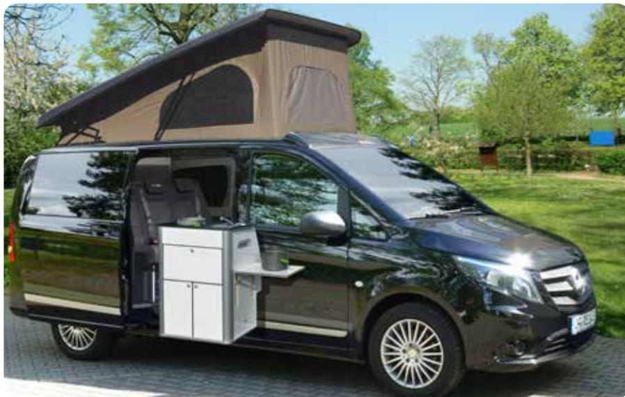
Swivel part for installation behind the passenger seat in the Mercedes Metris. The full bed length can be used in conjunction with a Reimo rock and roll bed V3000.
